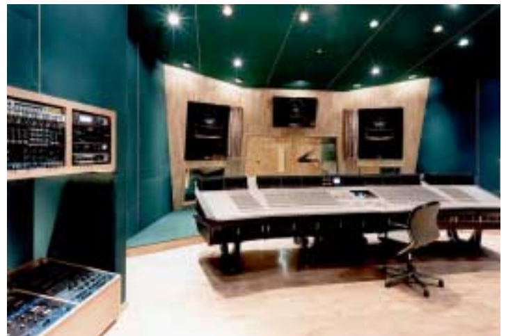
Masterfonics J (Nashville, USA 1996) 20 Hz Control Room was designed symmetrical also in vertical way with floor trap. It has extreme sound image by that.
