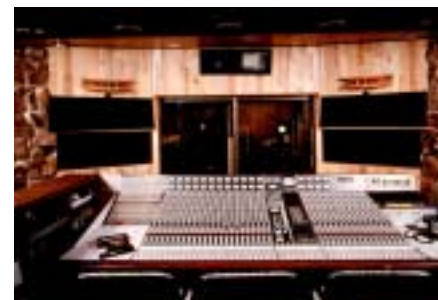
Ken Dun Studio (CA) around 1983. Designed by Tom Hidley. Monitor is of course by Hidley made. They used to be 3 way, and changed to 2 way after TD-4001, TL-1601a were introduced.
